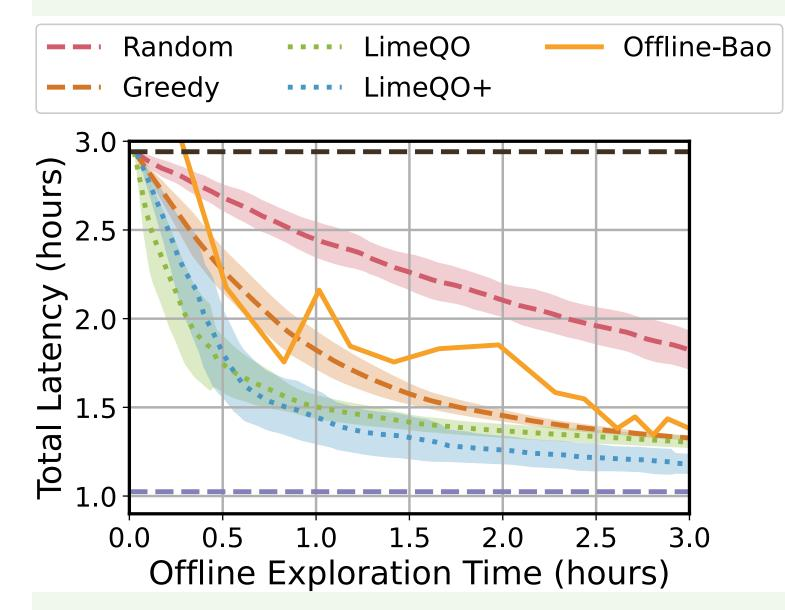
Caption: Both LimeQO and LimeQO+ outperform Bao Even without any features, pure linear method (LimeQO) can perform nearly as effective as the one using complex Neural Network (LimeQO+).
