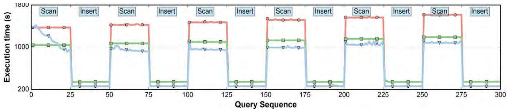
Figure 9: Workload-Aware Adaptation – The impact of tile group layout adaption on the query processing performance in an evolving workload mixture from the ADAPT benchmark. This experiment also examines the behavior of different storage managers while serving different query types in the workload.
