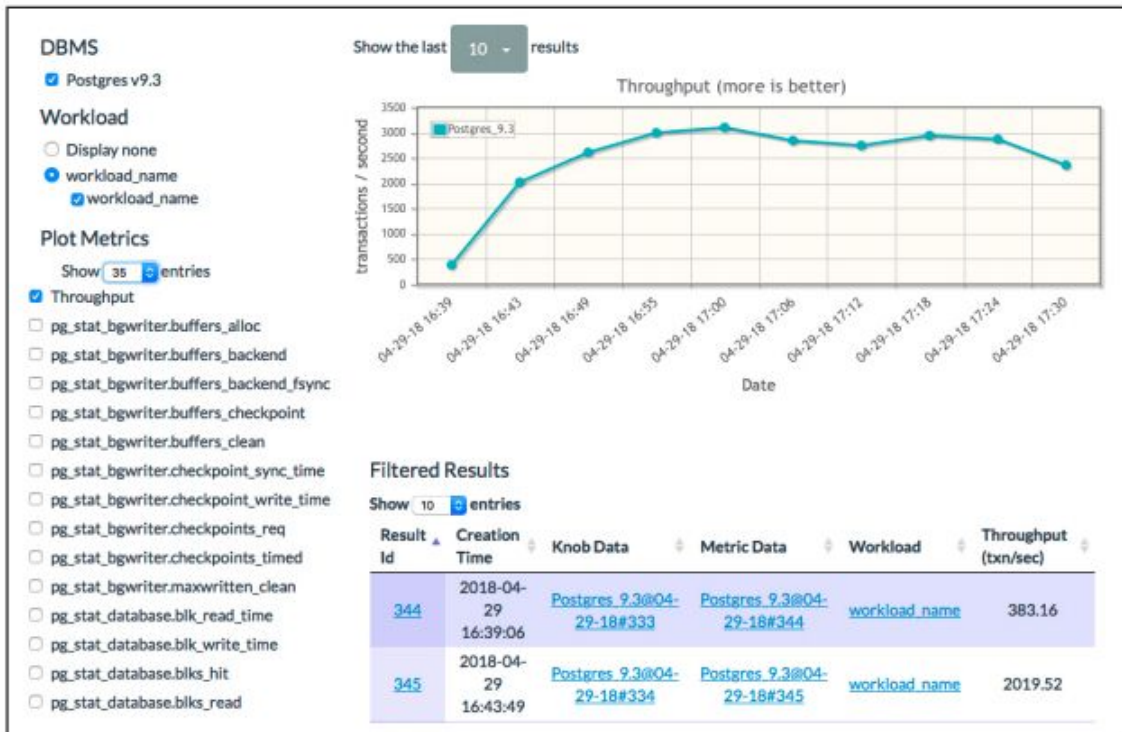
Figure 2: Tuning Session – The user can view the performance of the target DBMS as it tries the configurations recommended throughout the tuning session. Users can also view detailed information about the knob settings and metric values collected during each observation period.
